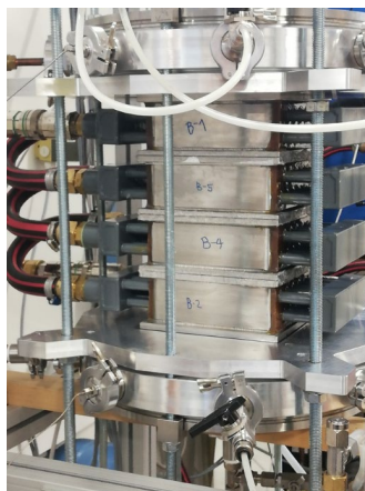
Figure 1. Flue gas separation column with inlet/outlet header flanges.
