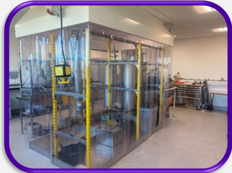
SMART Lab Rig at University of Sheffield (Frame - W:1.7m; L:2.7m; H:2.5m)
