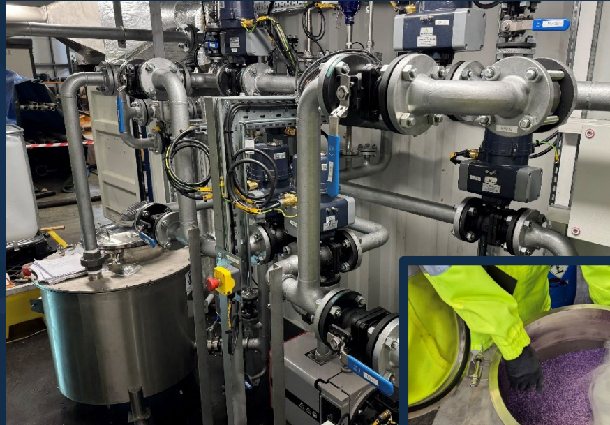
Promethean's pilot-scale carbon capture rig loaded with 50 kg of MOF
