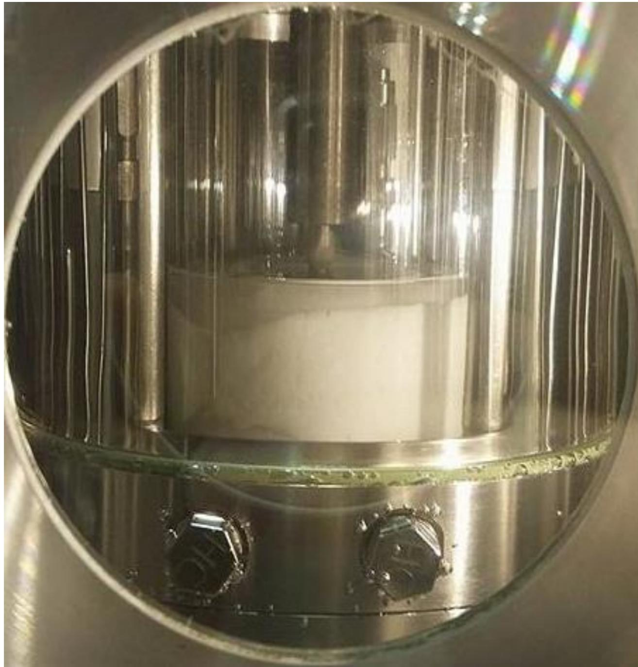
Experiments with 25 wt% AMP in TEGDME were cancelled because of severe precipitation and separation
