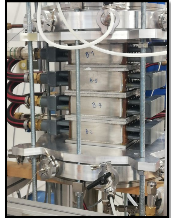
Flue gas separation column (OST)
