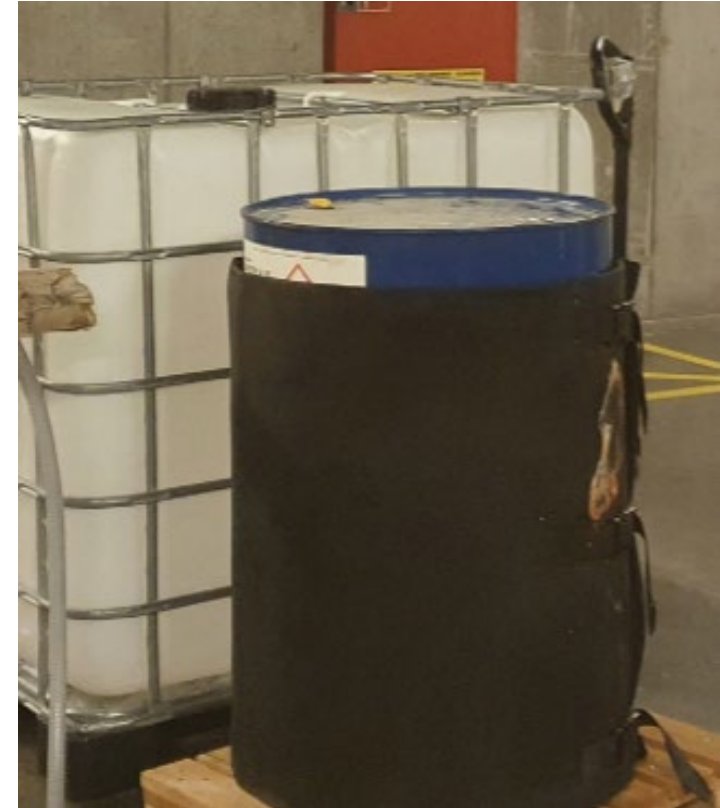
Heating jacket around the PZ barrel to maintain the liquid phase.
