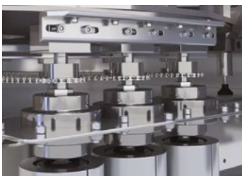
Patented external magnetic couplers drive the internal robotics
