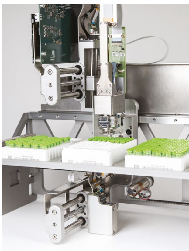
The Universal Picker provides the ability to pick multiple labware types with different diameters in one picker module
