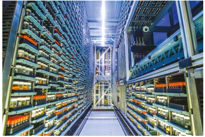
Tray shuttle robot to move the samples to the storage locations and tube picker inside Verso
