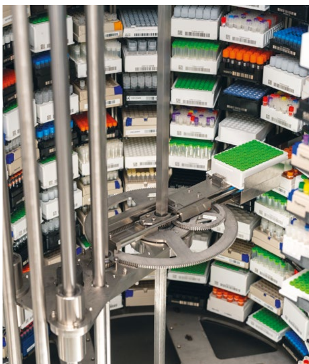
An internal carousel provides optimized and flexible storage capacities
