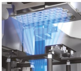
2D barcode scanning for full sample tracking
