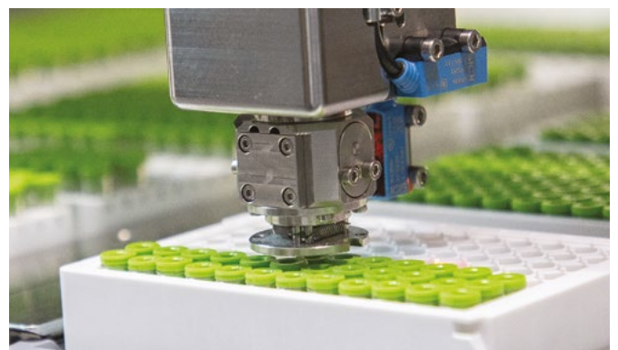
The Universal Picker provides the ability to pick multiple labware types with different diameters in one picker module
