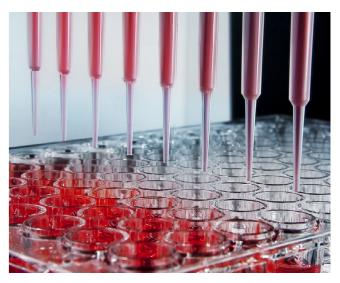
For CyBio® SELMA, using various types of microplates is simple and intuitive. In order to reach the optimum depth of tip immersion in each microplate well, the pipetting head can be brought into the right position thanks to an easy-to-use adjustment dial. For recurring processes, all adjustments such as dispense height, volume and pipetting speed are memorized, retrievable and changeable for regular use at any time.
