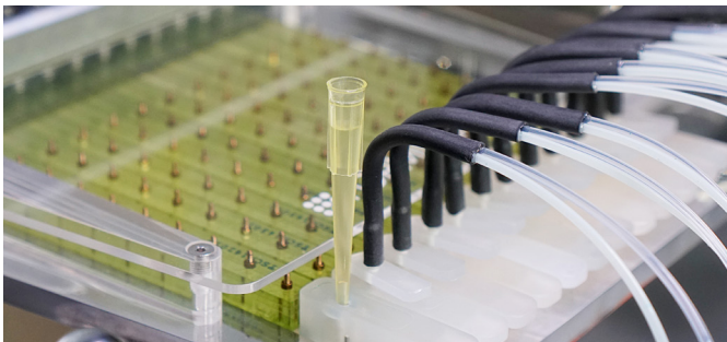
direct pipette tip dispenses reduce dead volumes of only 100 \mu L
