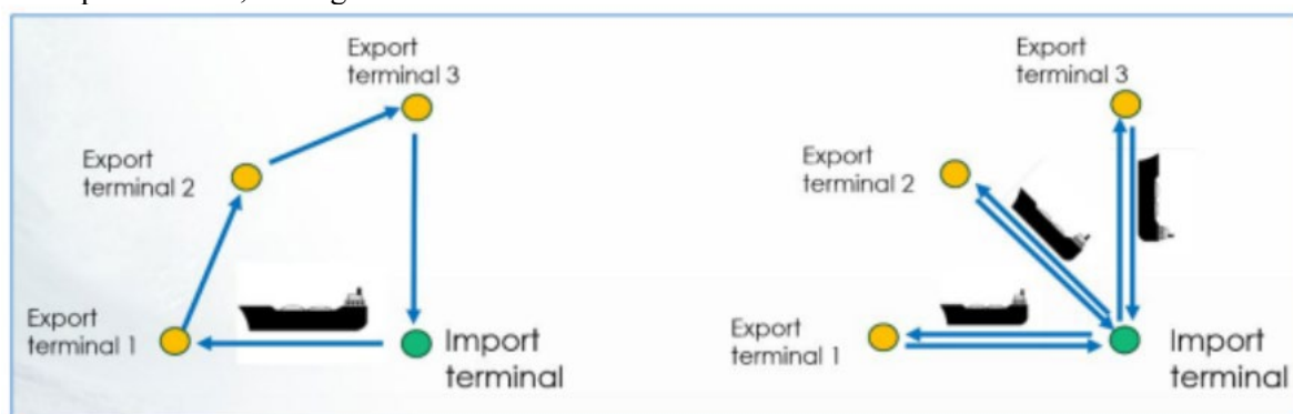
Figure 2: Co-loading (left) and Single loading (right)
