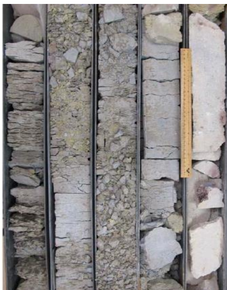
Figure 1 Picture of dehydrated and fractured caprock samples of N Field after being exposed air and humidity without proper preservation.
