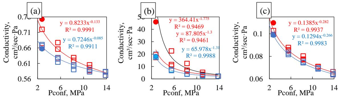
**Figure 3** Conductivity of a porous sandstone sample (a), a sample with an artificial crack (b) and a replica with a groove size of 350x150 μm (c) from the confining pressure. Red symbols correspond to the loading path, blue symbols - to the unloading path. Solid red and blue dots are the initial and final conductivity, respectively. Solid lines are approximations.
