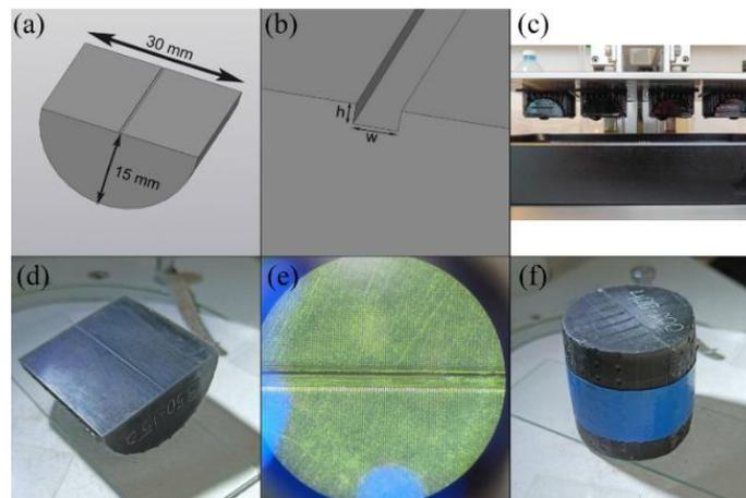
**Figure 1** Replicas fabrication: a – shape and size of the core half; b – shape of the groove; c – printing; g – the printed half; d – view of the groove under a microscope; e – replica assembled from two halves.
