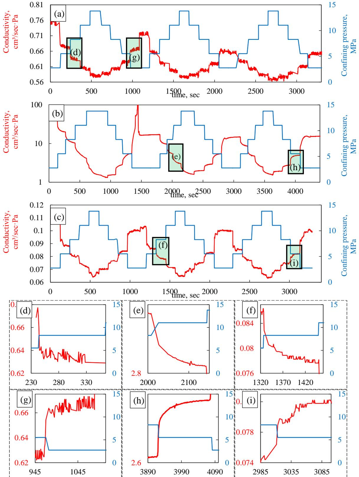
**Figure 2** Dynamics of conductivity of a porous sandstone sample (a, d, g), an impermeable sample with an artificial crack (b, e, h) and a replica with a groove size of  $350 \times 150 \mu\text{m}$  (c, f, i) under cyclic loading. The red line is conductivity, the blue line is the confining pressure.
