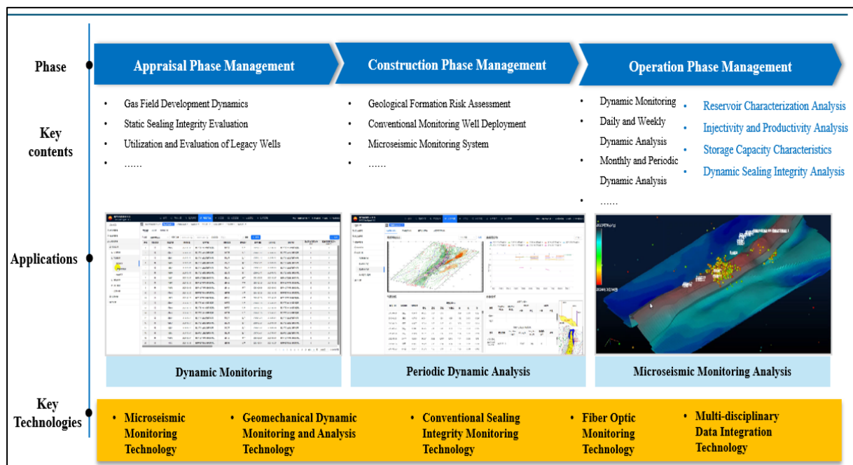
Figure-2, Phased Geological Reservoir Management with corresponding monitoring technologies integration to dynamically evaluate the sealing integrity of the Geobody, ensuring the gas storage formation remains safe and controllable
