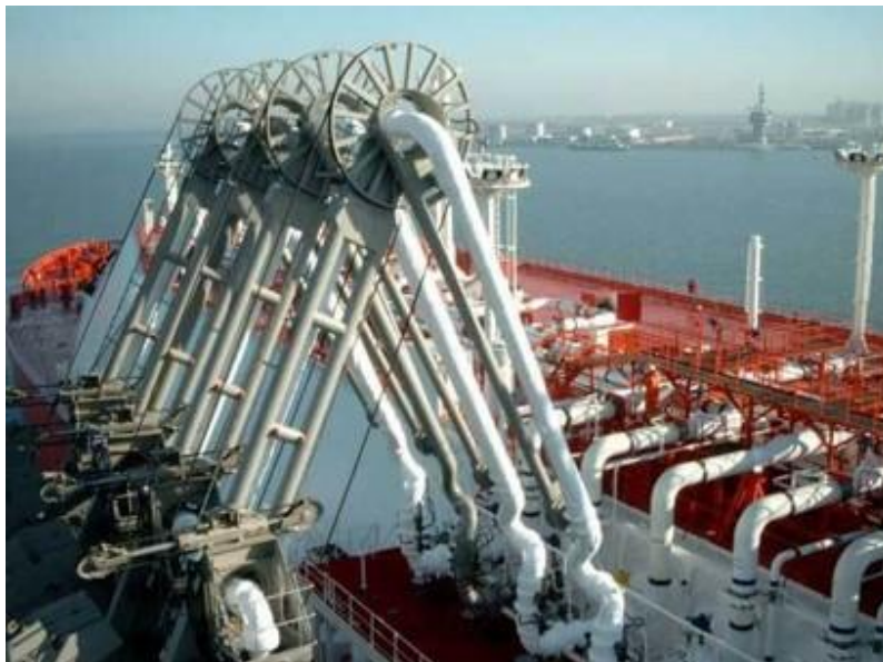
Figure 2 Example of a loading arm solution. (CONNEX SVT Inc., 2025)
