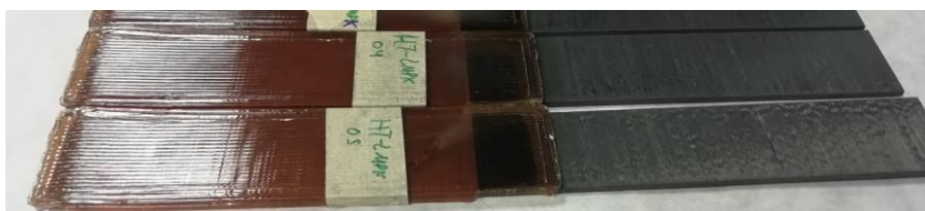
Figure 9: Single Lap Shear specimen manufactured by FFF.
