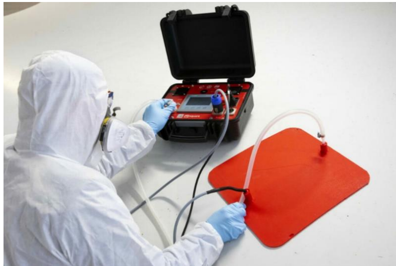
Figure 2: Heated blanket for induction welding in hard- patch repair.
