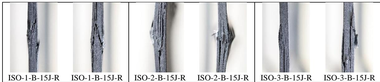
Figure 8: Comparison of fracture mechanisms for the 3 isotropic designs (ISO-1 – ISO-3) following bottom surface (B) impact of 15J using the standard rectangular aperture (R) impact fixture, viewed from the left and right side respectively.
