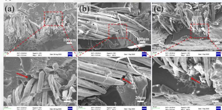
Fig. 5 Tensile fracture surface morphologies of (a) FY-RI, (b) FY-PI-UM, and (c) FY-PI-M. Red arrows indicate the interface between flax fibre yarn and PLA matrix.
