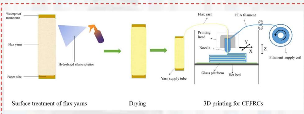
Fig.1 Schematic of fabrication process of 3D printing of CFRFCs.
