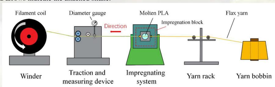
Fig.3 Schematic diagram of the fabrication process for pre-impregnated filaments.
