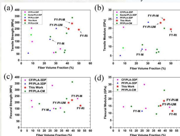
Fig.6 Comparison of mechanical properties of continuous fibre-reinforced PLA composites fabricated by 3D printing (3DP) and compression moulding (CM): (a-b) tensile properties, (c-d) flexural properties. PF represents plant fibre.
