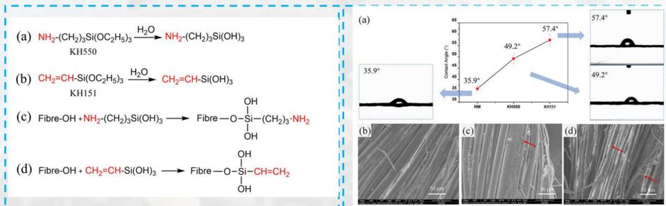
Fig.2 Left: Hydrolytic process of (a) silane KH550 and (b) silane KH151, and (c, d) condensation reaction between flax fibre and silanol. Right: (a) Measured contact angle and (b) surface morphologies of untreated, (c) KH550 treated and (d) KH151 treated flax yarns. The red arrows indicate the attached silane.
