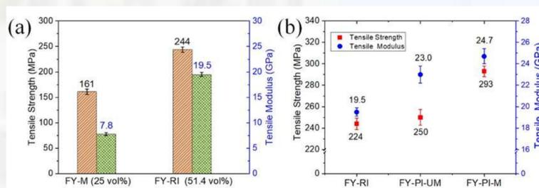
Fig.4 Tensile properties of (a) CFRFCs with different fibre volume fractions and (b) three types of CFRFCs
