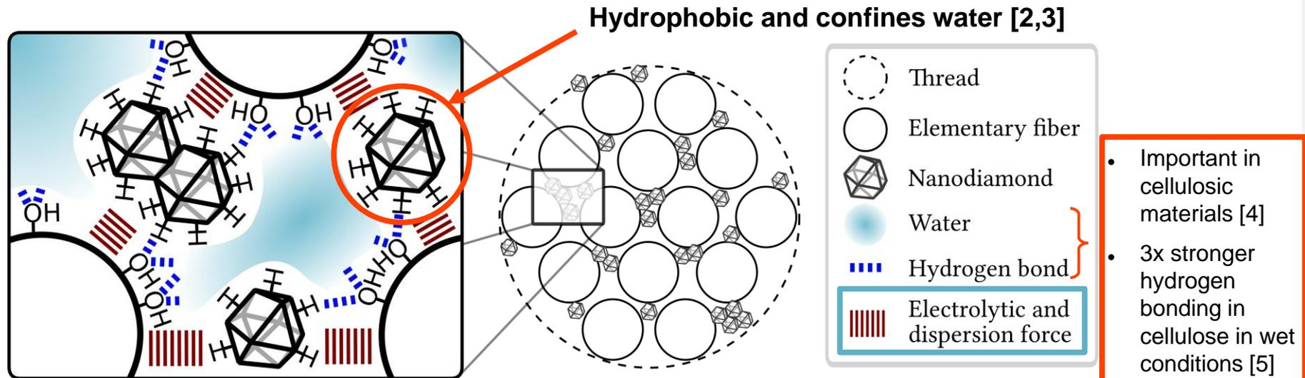
Fig. 15: Schematic (not to scale) of a thread's cross-section; Nanodiamonds bond between elementary fibers, increasing the adhesion between the elementary fibers and strengthening the thread; Additional water is confined by the hydrophobic nanodiamonds to further increase the adhesion between the elementary fibers [1]
