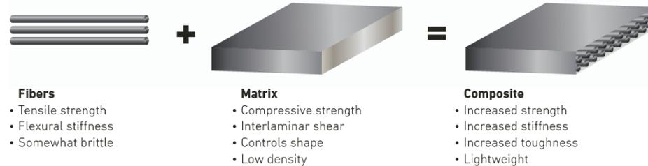
Fig. 1: Fiber reinforced composite material [1]
