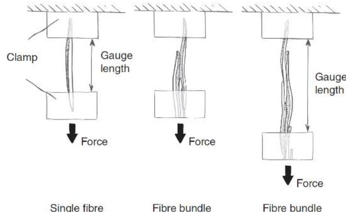
Fig. 12: Different clamping conditions [3]
