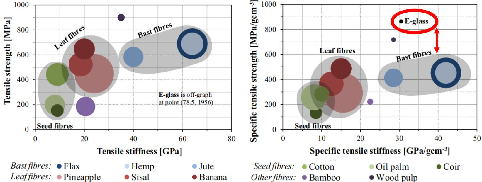
Fig. 4: Comparison of typical strength and stiffness performance of various plant fibers [1]
