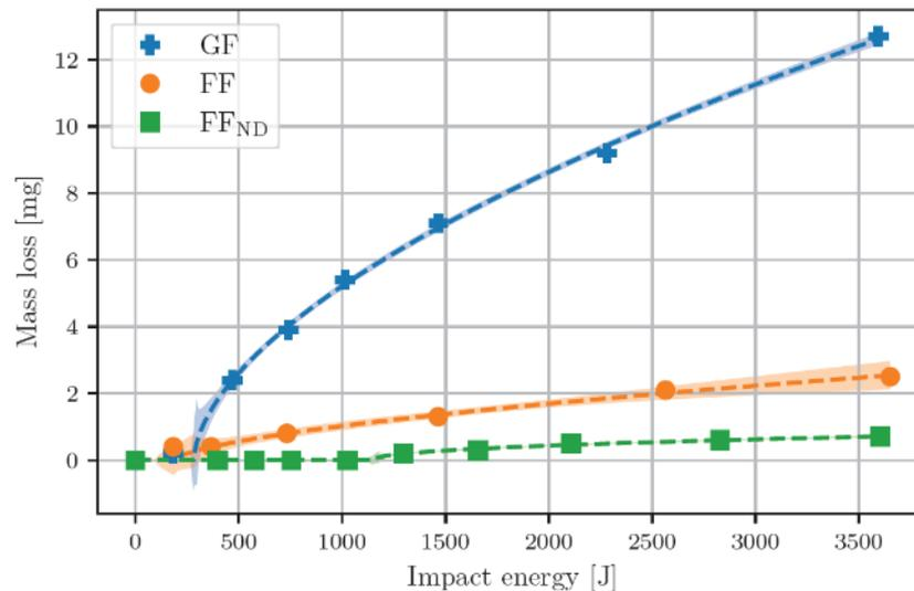
Fig. 18: Mass loss as a function of accumulated impact energy for impact velocities of  $160\text{m/s}$
