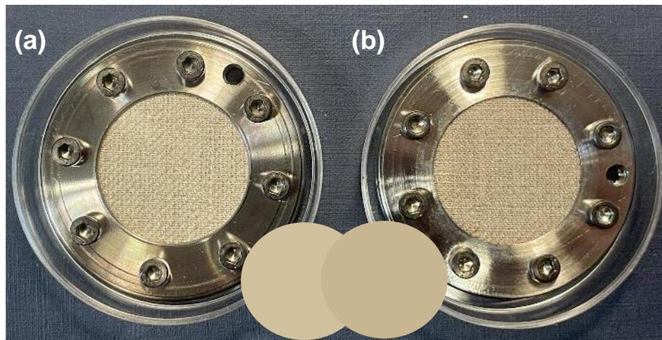
Fig. 7: White light image of untreated (a) and nanodiamond treated flax (b) [1]
