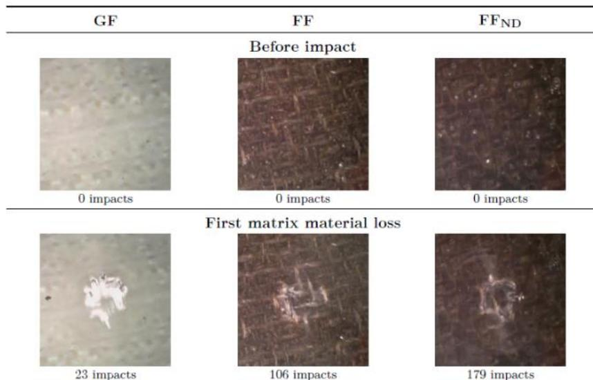
Fig. 17: Impact number to reach first matrix material loss ( $v = 160\text{m/s}$ )
