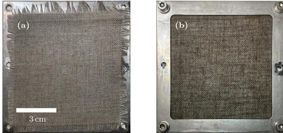
Fig. 6: Picture of dry flax fabric on base plate (a) and wet flax fabric mounted for treatment (b) [1]
