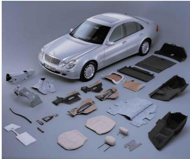
Fig. 2: Components of Mercedes E-Class from late 1990s using natural fiber composites [1]
