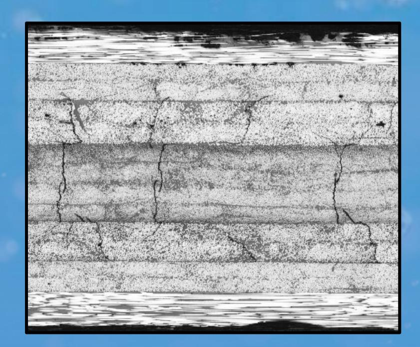
Typical Image of Microcracks in Composite Specimens, Layup  $[90_2/45_2/-45_2/0_2]_s$
