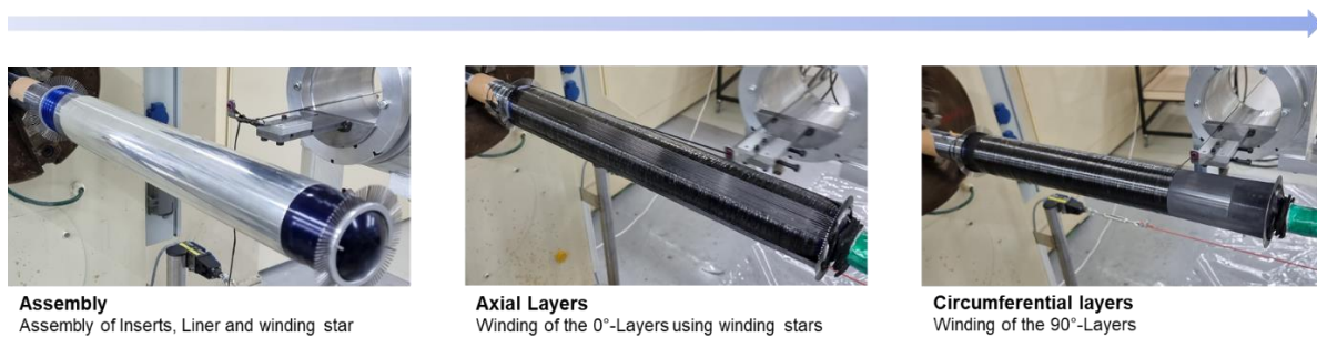
Figure 4: manufacturing process of the pressure vessel
