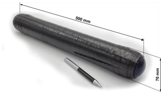
Figure 5: First Demonstrator for burst pressure test
