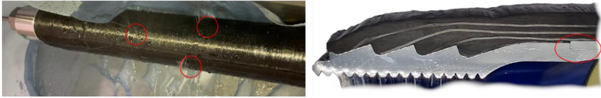
Figure 7: Burst pressure test of the pressure vessel
