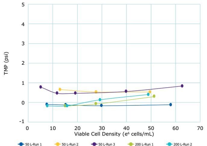
**Figures 2 and 3:** 50 L and 200 L Cellicon® filters demonstrate robust performance across separate runs, shown by consistent viable cell density (VCD), cell viability and transmembrane pressure (TMP) profiles. Each filter easily achieves target cell density for N-1 application with no filter fouling observed.
