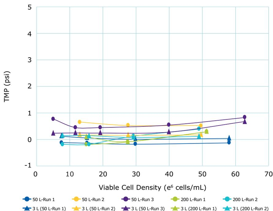
**Figure 4:** Similar fouling profiles were achieved between the Cellicon® 3 L and process-scale (50 L & 200 L) filters, demonstrating direct scalability while obtaining consistent cell growth. Maximum recommended TMP of 5 psi.
