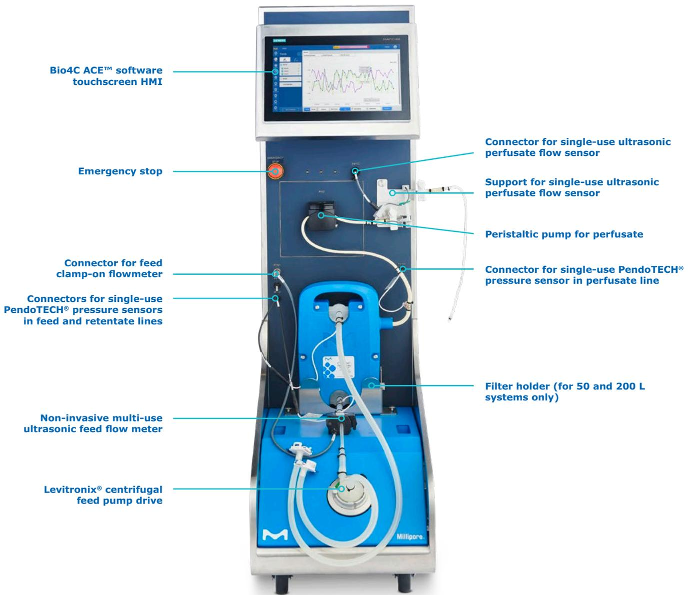
**Figure 6:** Mobius® Cell Retention System components
