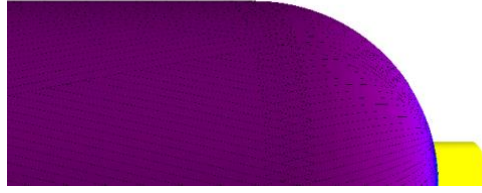
Figure 3. Tank wound at 13.2 degrees, using 145 circuit repeats, resulting in 100% fibre coverage.
