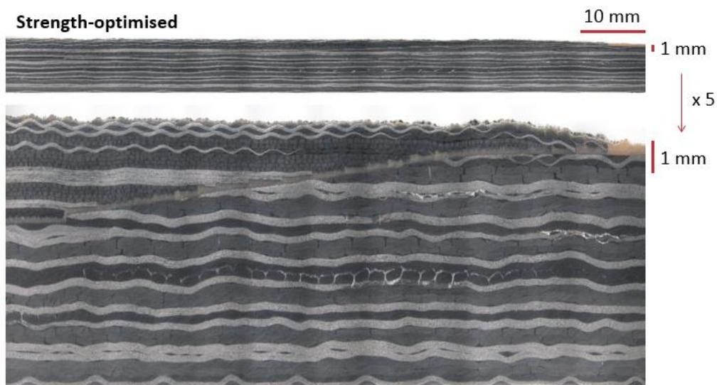
Figure 5: Strength-optimised scarf repair bond-line, including 5x height-stretched visualisation.
