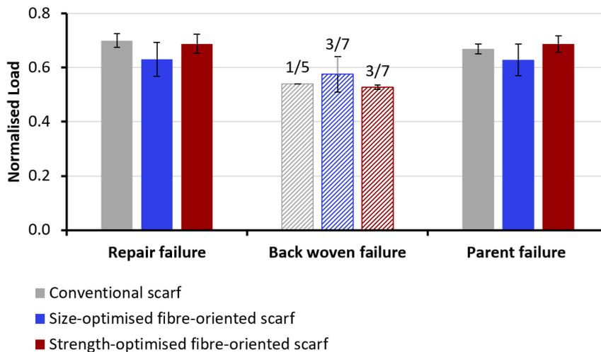
Figure 7: Normalised failure loads for the different repair configurations (related to the failure peaks in Figure 6). Back woven failure was only observed in a subset of the samples, as labelled.
