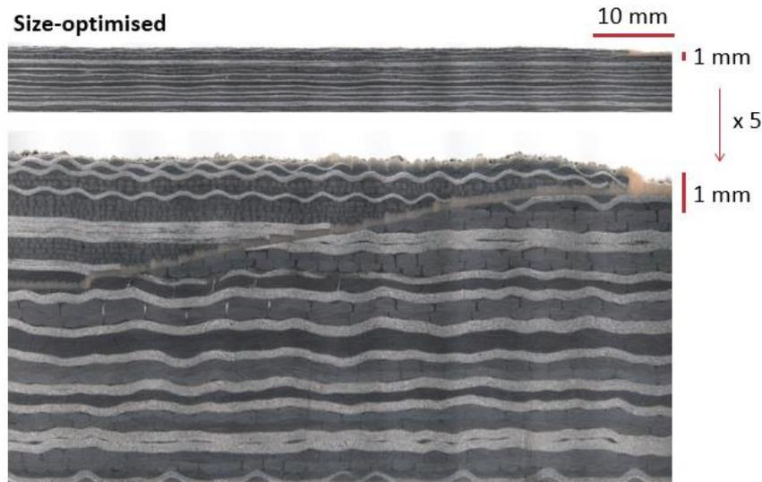
Figure 4: Size-optimised scarf repair bond-line, including 5x height-stretched visualisation.
