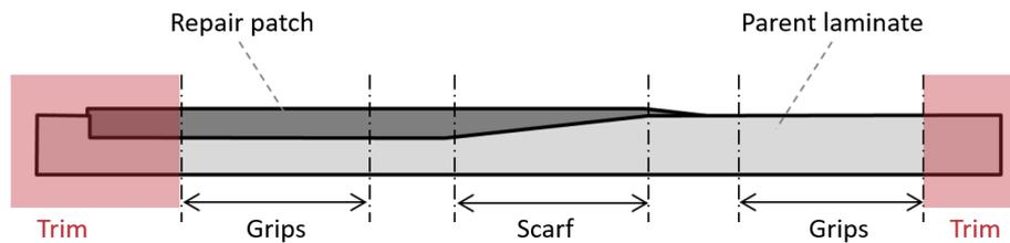
Figure 1: Scarf repair coupon configuration.
