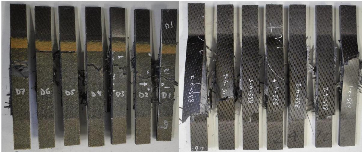
Figure 8: Front (left) and back (right) surfaces of the failed size-optimised fibre-oriented scarf repair.
