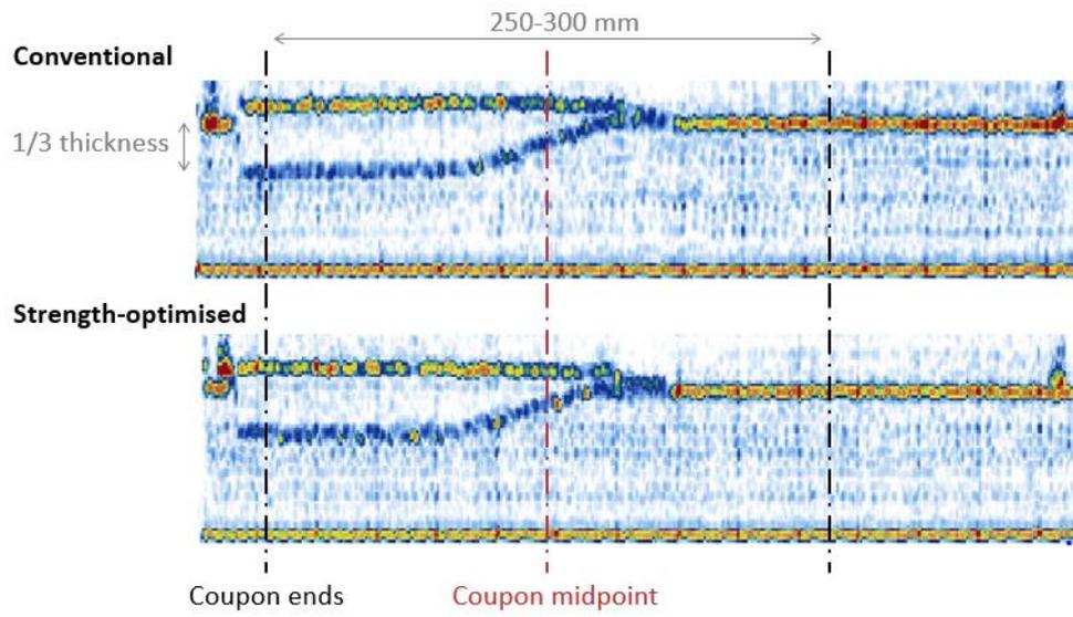
Figure 2: Representative ultrasonic B-scans of conventional and strength-optimized repairs.
