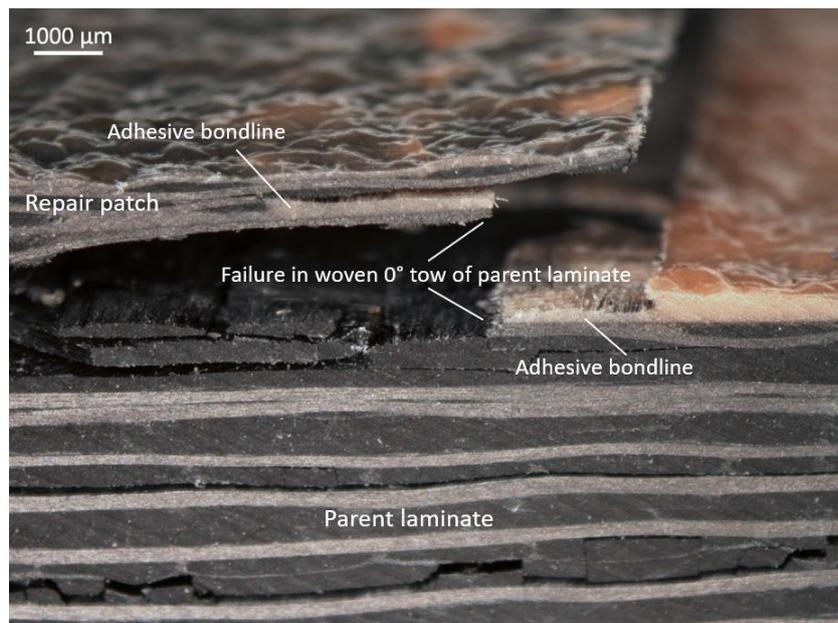
Figure 9: Microscopy of first failure, initiated by exterior woven ply of parent laminate.
