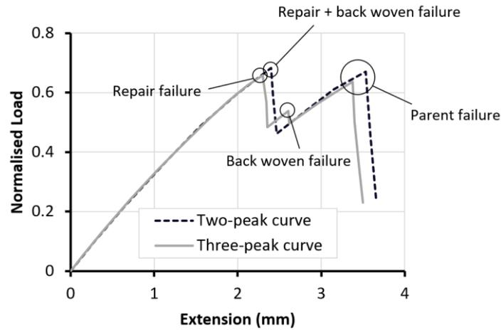
Figure 6: Normalised tensile load-extension curves for the two behaviours representative of all repair coupons.
