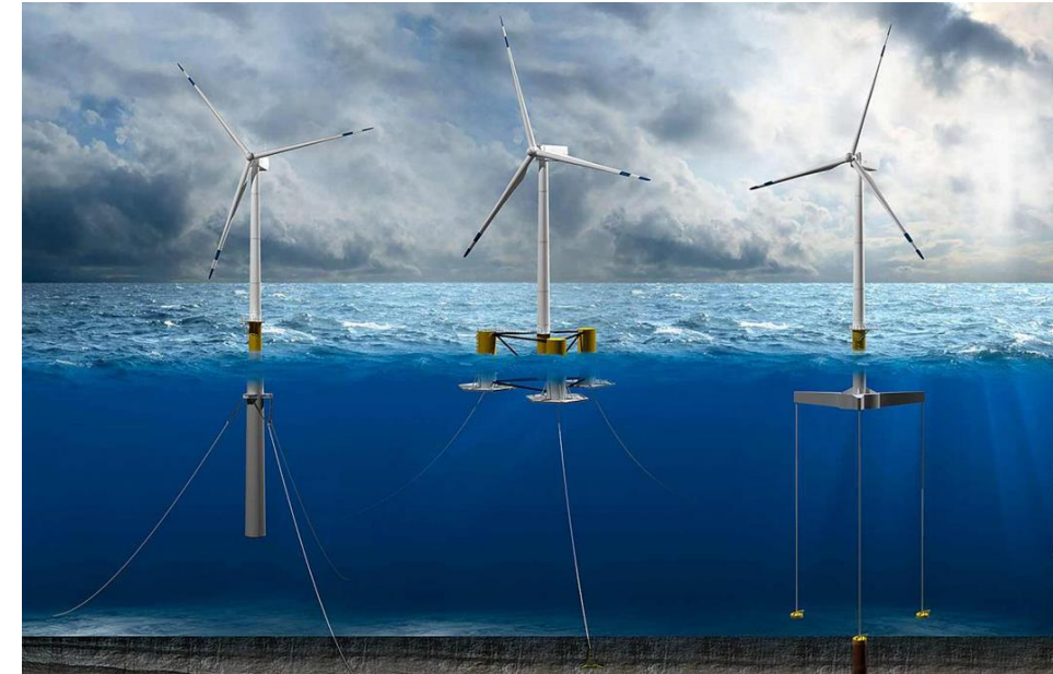
Floating Horizontal axis wind turbine [2]
