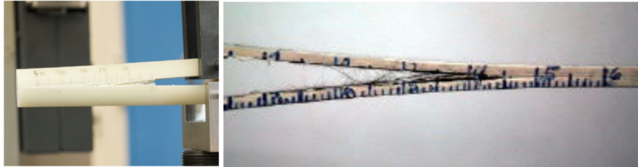
Figure 1: Mode I tensile opening fracture tests on (left) glass-fiber reinforced rod with unidirectional fiber lay-up yielding significant fiber bridging and delamination resistance (right) carbon-fiber reinforced laminate beam also with large-scale fiber bridging, but to a much lesser extent.
