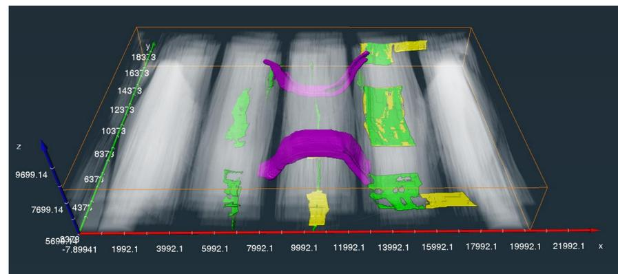
Figure 4, the 3D volume rendering showing the global cracks distribution of the sample after 5000 cycles loading. ( For easier reading, only weft bundles (white) and part of the Z-binder (Purple) are rendered.) Green: Debonding; Yellow: Delamination.
