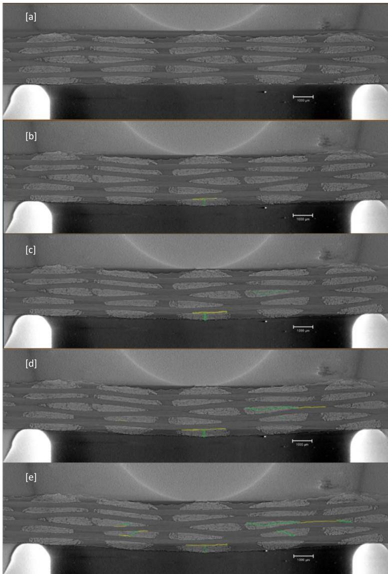
Figure 3, progressive fatigue damage development morphologies of the SBS specimen at different stages of fatigue loading: [a] reference imaging, [b] 1000 cycles, [c] 2000 cycles, [d] 3000 cycles, [e] 5000 cycles. Green: Debonding; Yellow: Delamination
