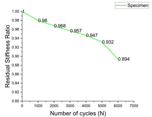
Figure 2, the Stiffness reduction was monitored and recorded using Instron 8801 hydraulic test machine
