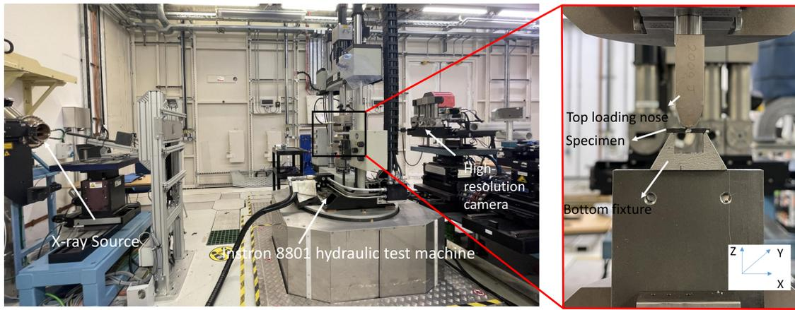
Figure 1, Photograph of the experimental set-up on the I-12 beamline at Diamond Light Source, showing the short beam shear fatigue loading of the composite by Instron 8801 in the sample stage, the details of samples set-up can be seen in the magnified insert.
