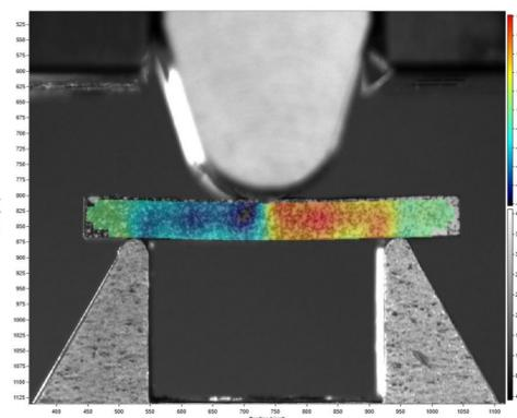
Figure 5, Full Field strain distributions measured by DIC
