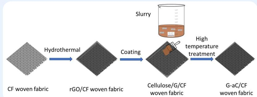
Figure 3 - Schematic of process steps to prepare G-aC/CF fabrics.
