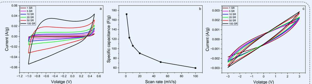
Figure 5 - Cyclic voltammograms a) CV curves for G-aC/CF, b) specific capacitance (C) values at different scan rates, c) CV curves for SSC device.
