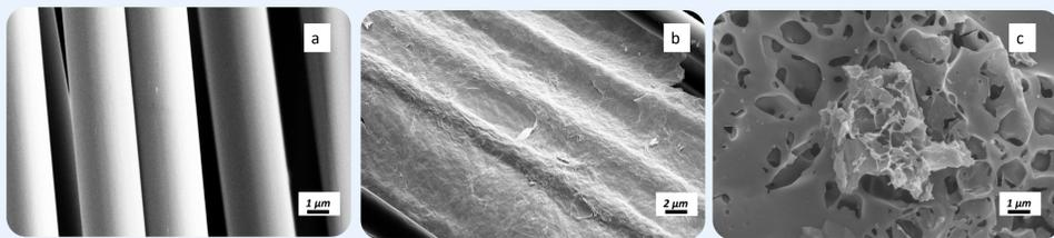
Figure 4 - SEM images of desized a) CFs, b) rGO/CF and c) G-aC/CF.
