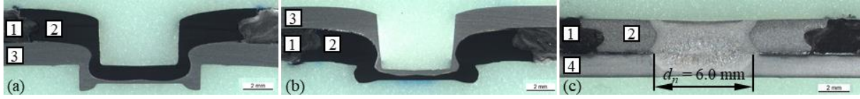
Figure 9: Micrographs of clinched and welded joints using the same insert geometry: (a) Clinching with insert punch sided, (b) clinching with insert die sided and (c) RSW (1: GF-PP, 2: S235JR, 3: EN AW-6016 T4, 4: HC340LA) according to [30]
