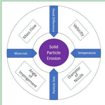
Figure - 2. Erosion Parameters
