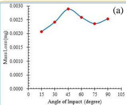
(a). Cumulative mass loss with respect to different impact angles.
