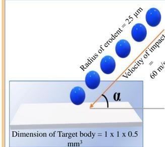
Figure - 8. Composite Model for Erosion Modeling
