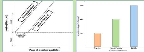
Figure - 3. Typical behaviour of Erosion
