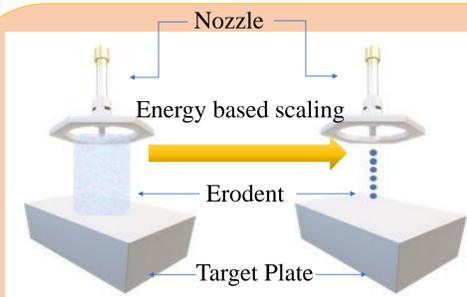
Figure - 6. Scaling of Eroder's for Erosion modeling
