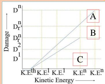
Figure - 7. Plot showing proportionality between damage & kinetic energy
