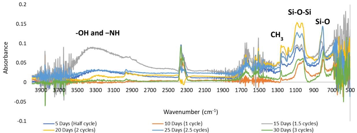
Figure 11. FTIR observation on liquid phase condition after exposure to cyclic solution concentration
