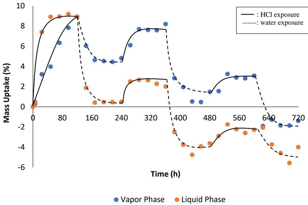
Figure 5. Mass uptake of glass fiber epoxy specimen in 35 mass% HCl and 0 mass% (water) under cyclic solution concentration
