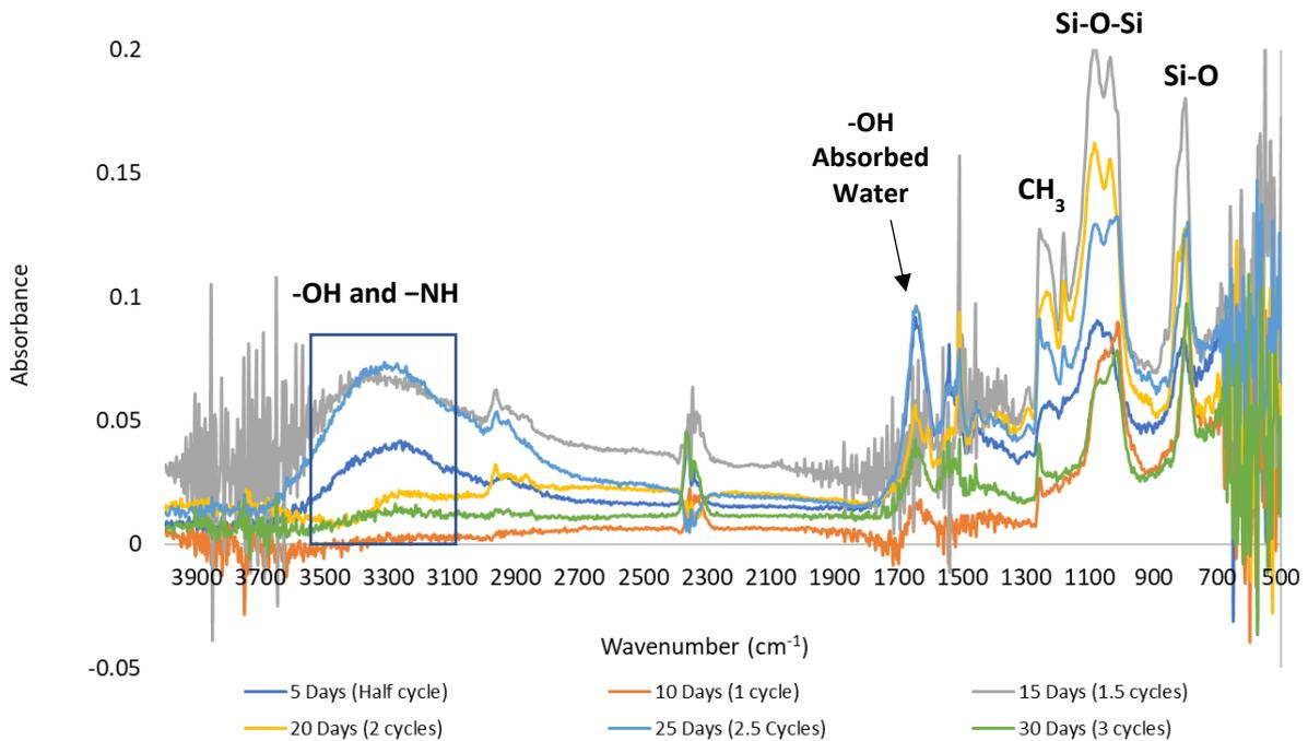
Figure 10. FTIR observation on vapor phase condition after exposure to cyclic solution concentration
