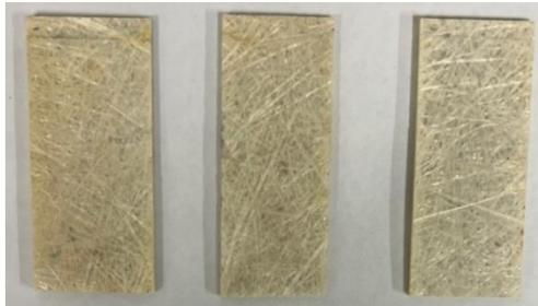
Figure 1. Final specimen of glass-fiber epoxy
