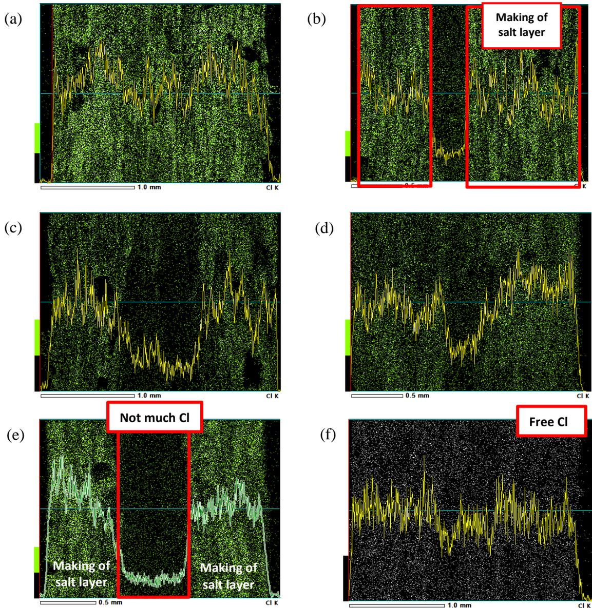
Figure 8. EDS Cl mapping of cross section glass-fiber-epoxy specimen in (a) vapor phase after 1 cycle (b) liquid phase after 1 cycle (c) vapor phase after 2 cycles (d) liquid phase after 2 cycles (e) vapor phase after 3 cycles (f) liquid phase after 3 cycles.
