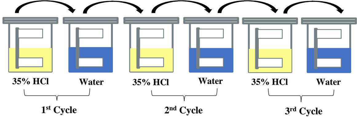
Figure 4. Schematic of cyclic solution concentration
