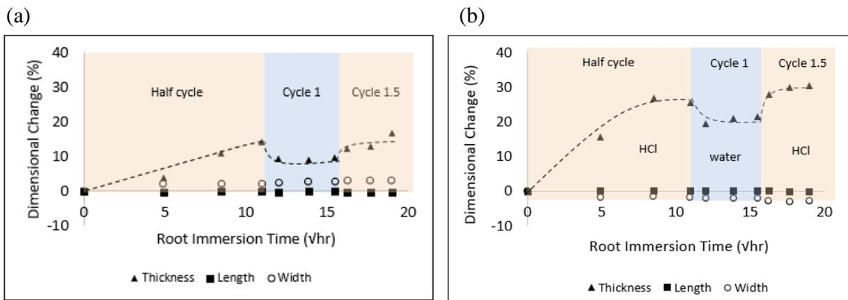
Figure 6. Dimensional change of glass fiber epoxy specimen in 35 mass% HCl and 0 mass% (water) under cyclic solution concentration at (a) vapor phase condition (b) Liquid phase condition
