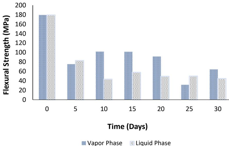
Figure 7. Flexural strength of glass-fiber-epoxy specimen in 35 mass% and 0 mass% (water) under cyclic solution concentration
