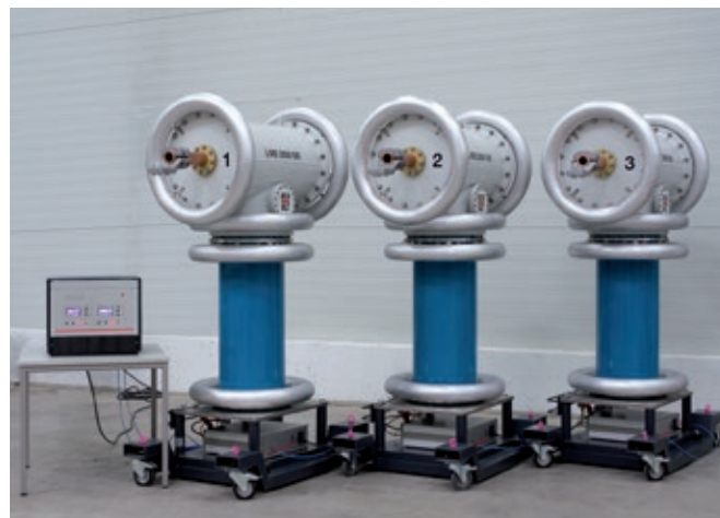
Fig. 4 Test system for large power transformers (left: 2 MW 4 MVA [SFC], tapped transformer and filters, right: loss measuring system LiMOS 2000/100-3)
