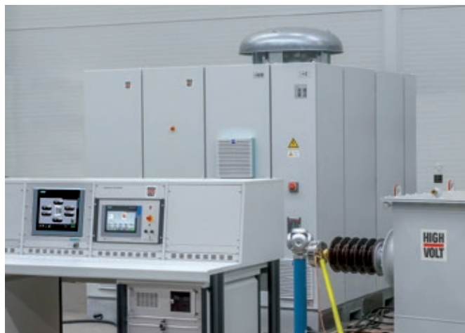
Fig. 1 Test system for type- and routine tests on distribution transformers (left: test voltage source and control system, right: automatic switching system)
