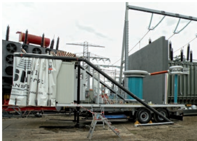
Fig. 4 Test system for on-site tests on transformers (left: WV 620-1000/80, right: extension for applied voltage tests WRV 5/360 M)
