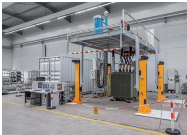
Fig. 1 Test system for type- and routine tests on distribution transformers (left: test voltage source and control system, right: automatic switching system)
