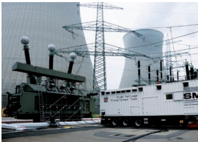
Fig. 4 Test system for on-site tests on transformers (left: WV 620-1000/80, right: extension for applied voltage tests WRV 5/360 M)
