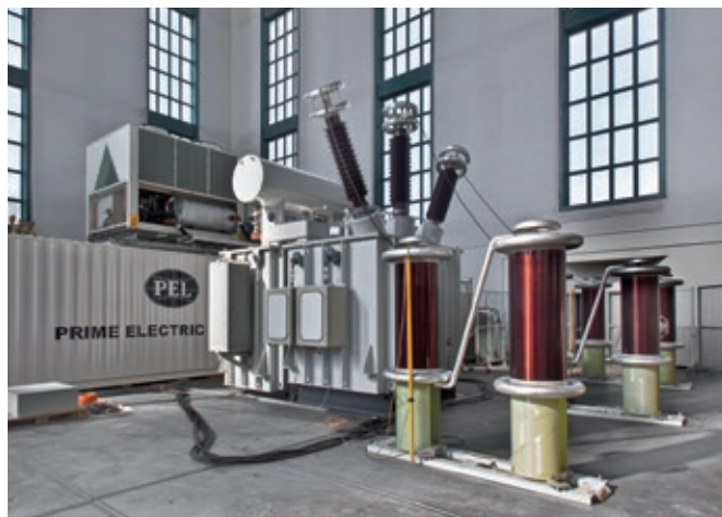
Fig. 4 Test system for large power transformers (left: 2 MW 4 MVA [SFC], tapped transformer and filters, right: loss measuring system LiMOS 2000/100-3)
