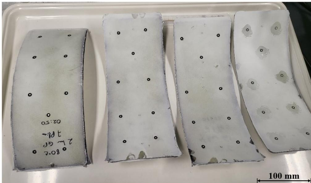
Figure 8: Manufactured experimental parts coated with SKD-2 solvent-based powder.
