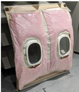
Figure 1 – Example of a sidewall with a conventional secondary insulation
