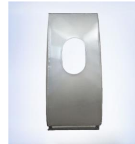
Figure 3 – Sidewall with attached Vacuum Insulation Panel
