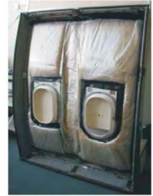
Figure 8 – Sidewall with secondary insulation on test rig [1]
