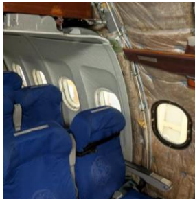
Figure 1 – Example of a sidewall with a conventional secondary insulation
