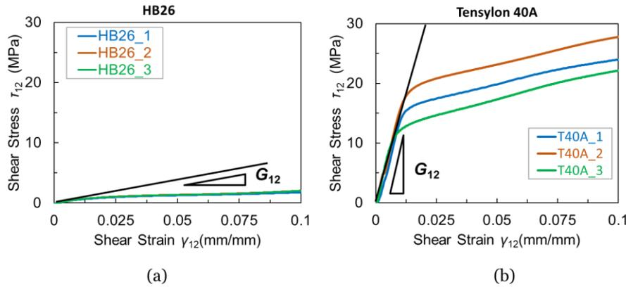
Figure 7: (a) Dyneema HB26 and (b) Tensylon HSBD 40A shear stress ( $\tau_{12}$ ) as a function of shear strain ( $\gamma_{12}$ )
