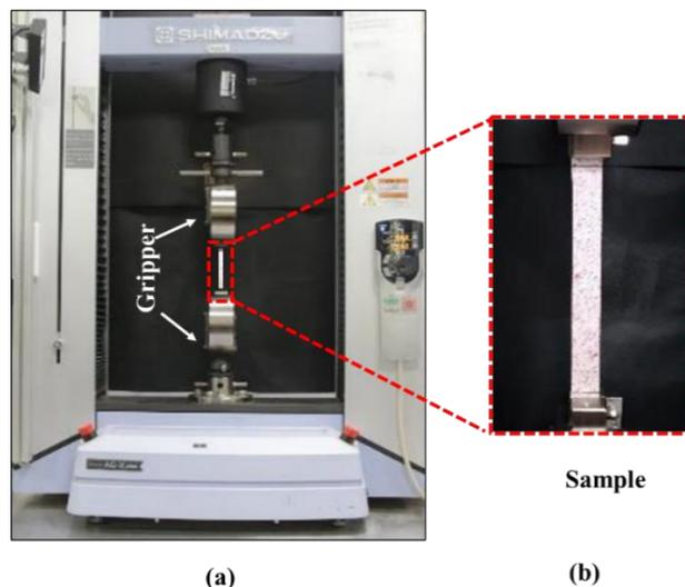
Figure 3: (a) Experimental setup, and (b) Sample clamped between grippers
