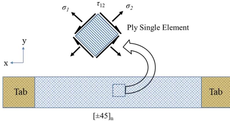
Figure 4: Schematic representation of tensile test sample with orientation and stress state
