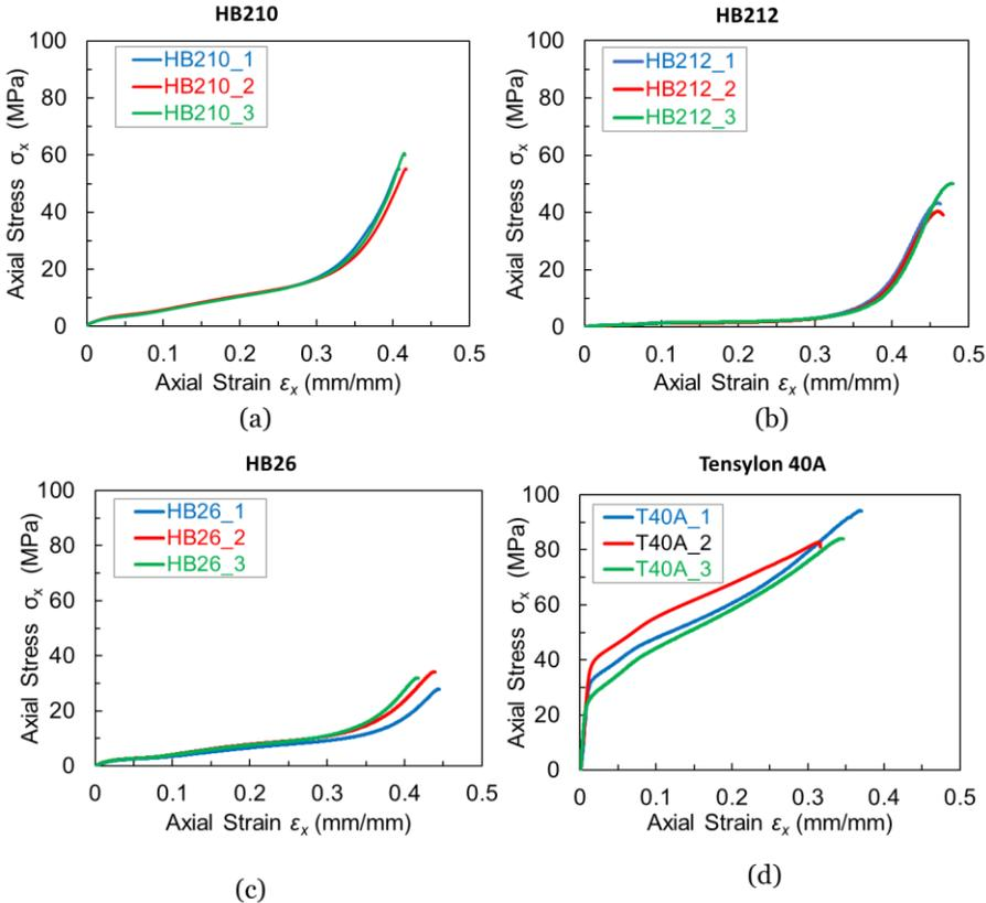
Figure 6: Axial engineering stress ( $\sigma_x$ ) with respect to axial engineering strain ( $\epsilon_x$ ) for (a) Dyneema HB210, (b) Dyneema HB212, (c) Tensylon HSD 40A, and (d) Dyneema HB26
