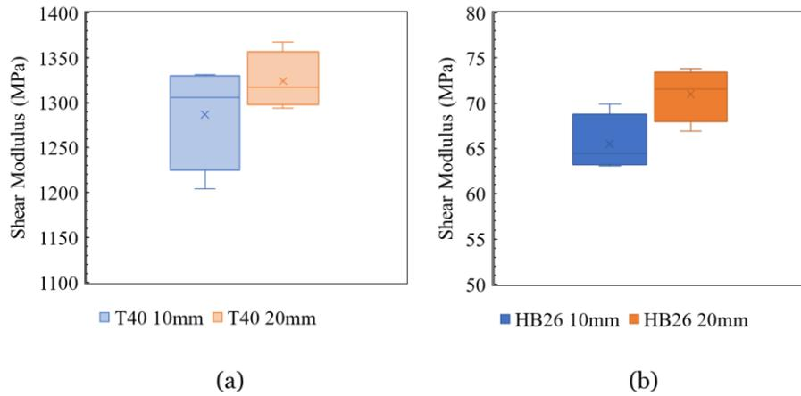
Figure 8: Tensylon HSB40A and Dyneema HB26 shear modulus ( $G_{12}$ ) with (a) 20mm and (b) 10mm width specimen
