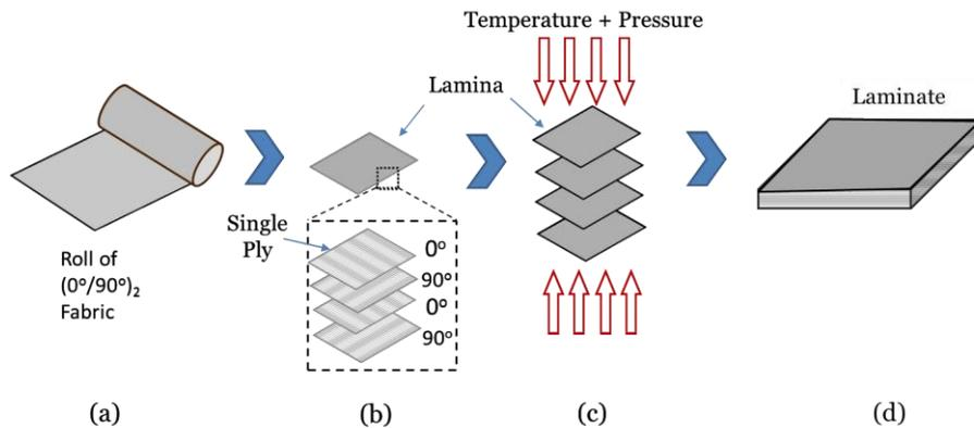
Figure 2: Steps for preparation of UHMWPE laminate
