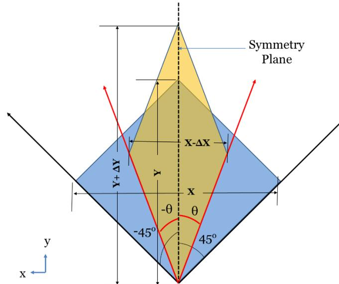
Figure 9: Fiber angle changes with applied load in the y-direction
