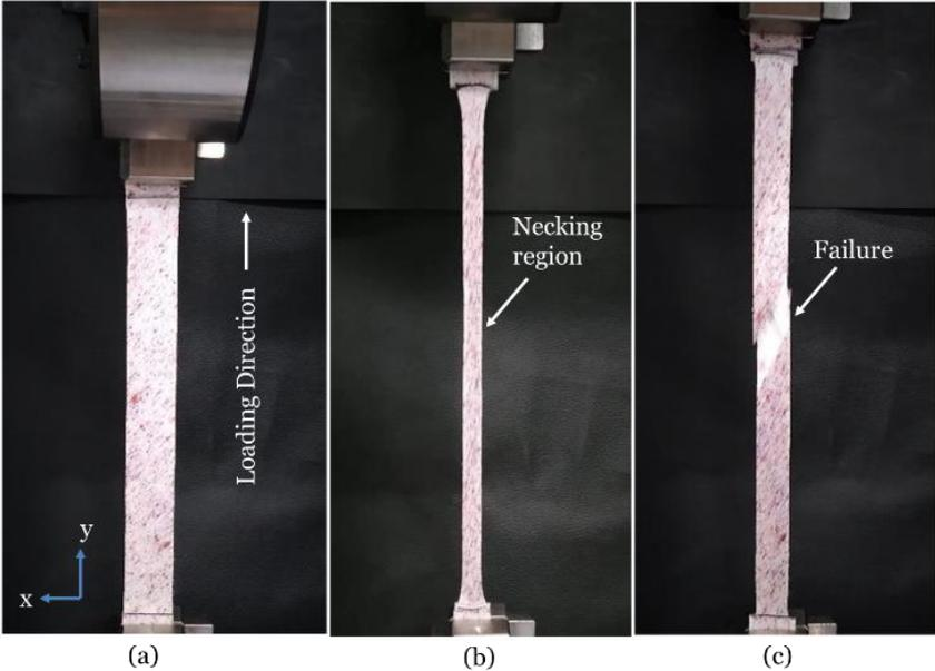
Figure 5: Dyneema HB210 specimen with eight plies (a) before load application, (b) just before failure, and (c) after the failure
