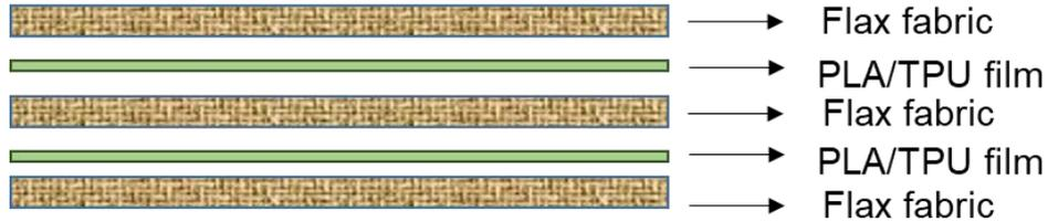
Figure 1a. Organosheet construction for the DVS measurement
