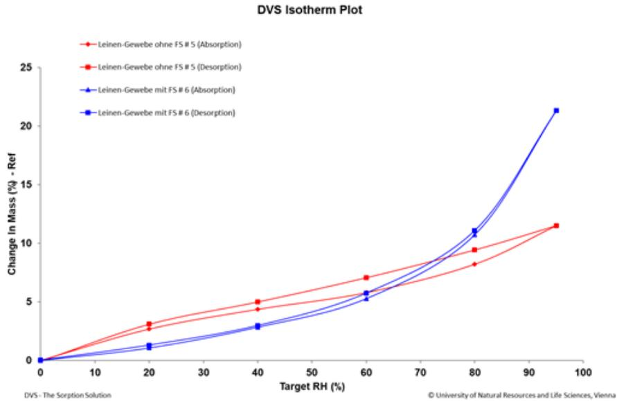
Figure 3. Absorption isotherms of flax fabric without (red) and with loaded flame retardant (blue)
