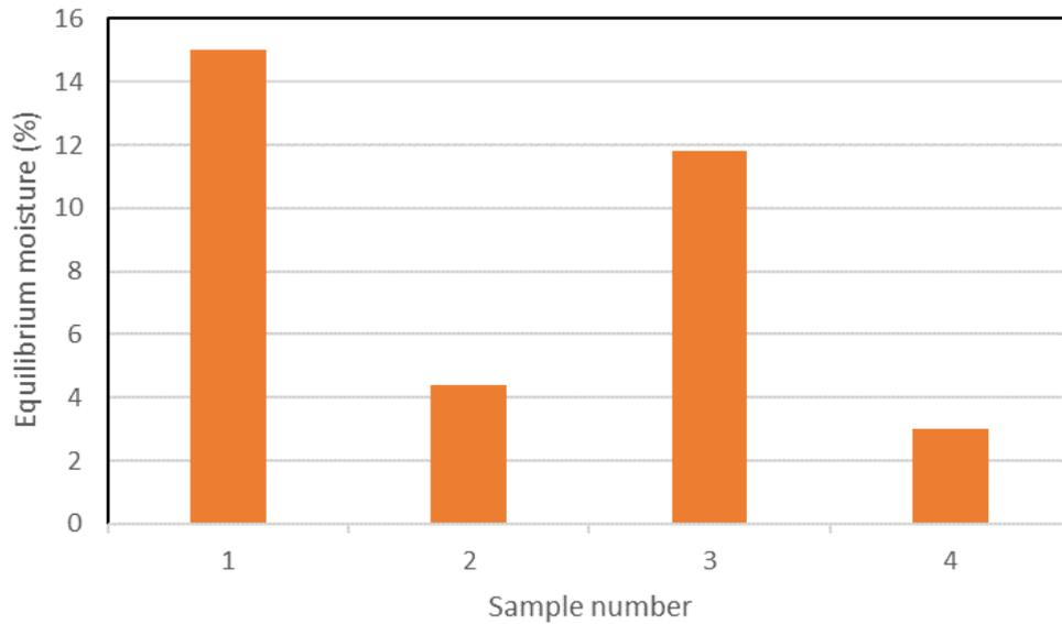
Figure 2. Change in moisture absorption measured using DVS instrument for different organosheet samples
