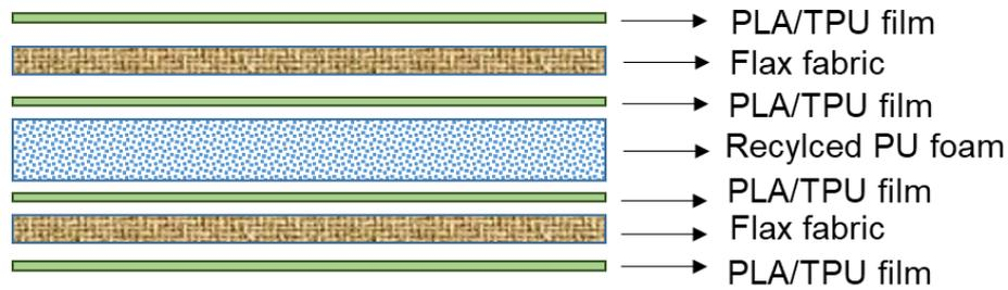
Figure 1b. Laminates with recycled PU foam core for flame retardancy test
