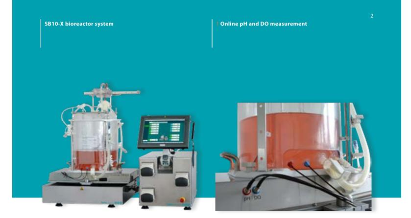
The SB10-X is an orbital shaken benchtop bioreactor system for the cultivation of human, mammalian and plant cells in a single-use bag. It consists of six modules (excluding the bag) and has a working volume from 4 litres up to 12 litres. The SB10-X can be used in research, process development or as a pilot scale bioreactor.
