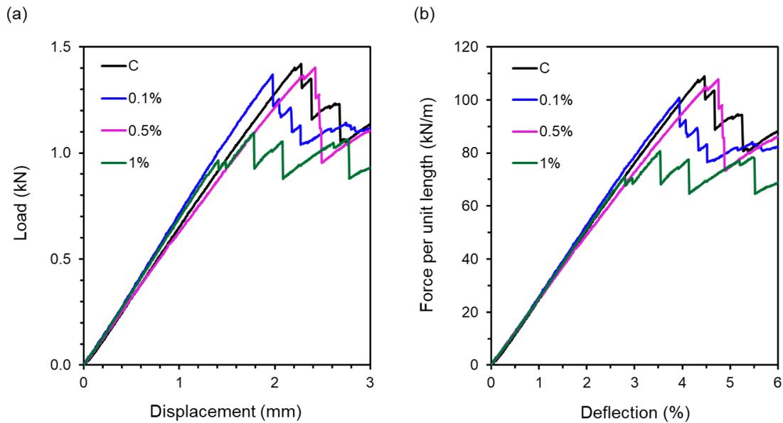
Figure 5: (a) Load-displacement curves and (b) force per unit length-deflection curves of the CFRP composite rings with different GNP loadings under radial compression.
