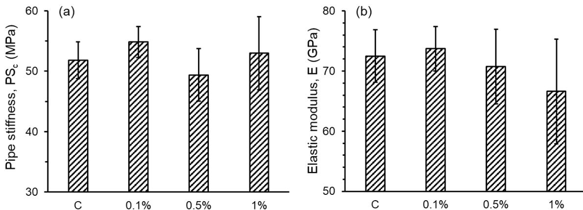
Figure 6: (a) Corrected pipe stiffness ( $PS_c$ ) and (b) elastic modulus ( $E$ ) of the composite rings under radial compression, considering both 2.5% deflection and failure point conditions.
