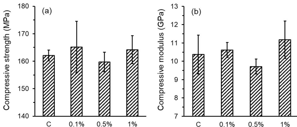
Figure 4: Axial compressive (a) strength and (b) modulus of the composite rings with different GNP loadings.
