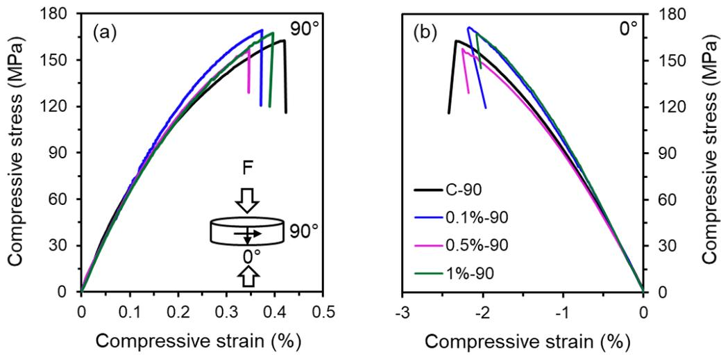
Figure 3: Stress-strain curves of the CFRP composite rings with different GNP loadings under axial compression, at both (a) transverse (90°) and (b) longitudinal (0°) directions.
