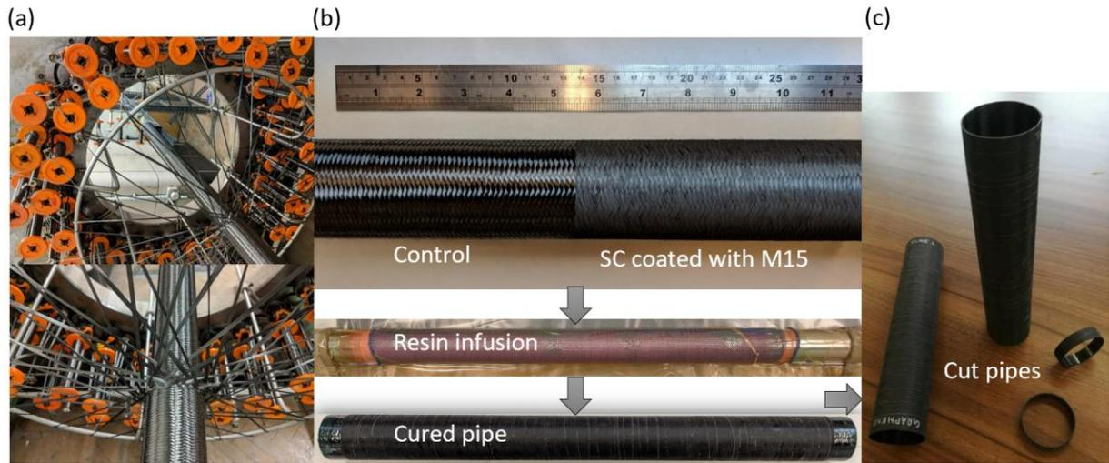
Figure 1: Images of the (a) carbon fibre braiding procedure; (b) composite pipe fabricated by vacuum assisted resin infusion (VARI); (c) cured pipes and cut rings.
