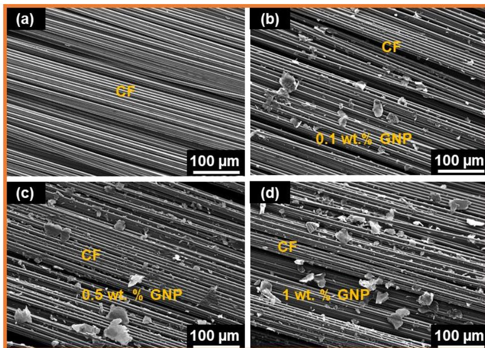
Figure 2: (a-d) SEM images of carbon fibres spray coated with 0, 0.1 wt. %, 0.5 wt. % and 1 wt. % GNPs.
