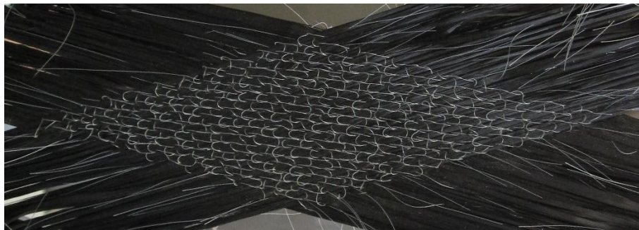
Figure 4: Sheared textile sample during the picture frame test.
