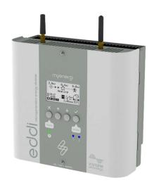
eddi is an eco-smart energy management system. It diverts surplus power from solar PV or wind generation to a designated heating appliance such as an immersion heater. This excess energy will go directly to the appliance (or two sequentially). eddi allows you to stop exporting surplus energy back to the grid and saves you money on your energy bill.
