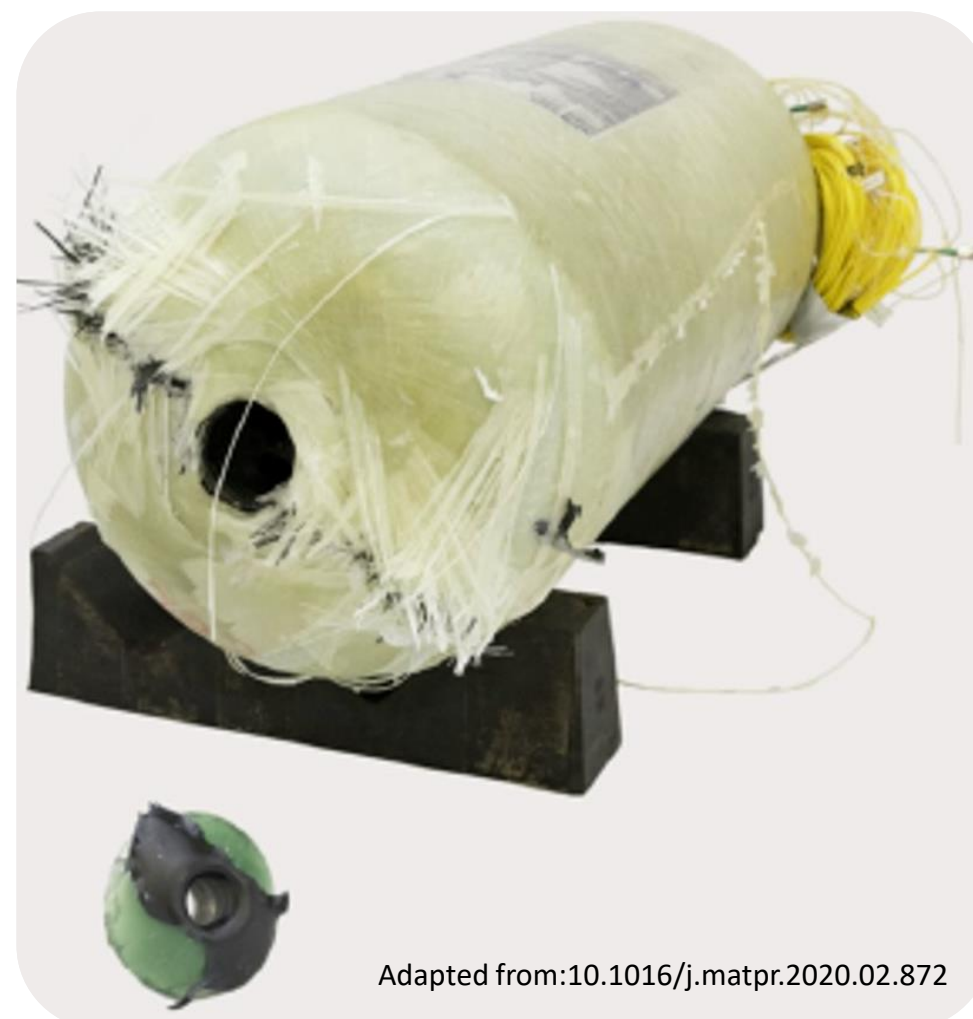
Fig. 4 Catastrophic Failure of Boss
