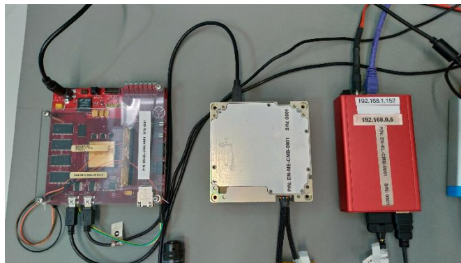
Figure 3 Hardware in the loop setup
