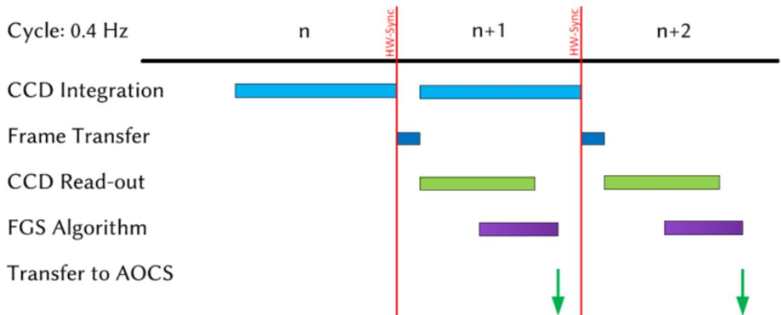
Figure 5-26: Fine Guidance Data Transfer Timeline
