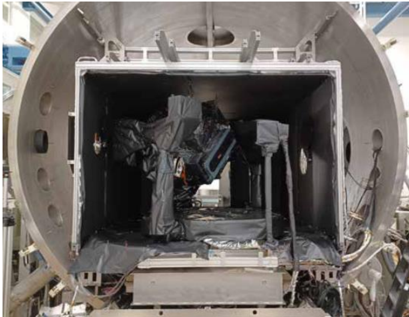
Figure 8: The instrument mounted on the turning table inside the thermal tent inside the vacuum chamber at CSL.
