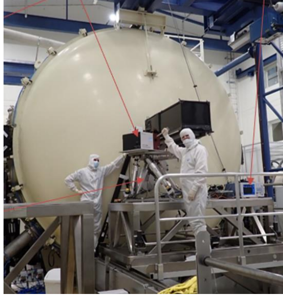
Figure 3: The ISRF OGSE mounted in front of the 5m vacuum chamber. The larger black box in the centre of the vacuum chamber lid contains the filter, the integrating sphere and the off-axis parabola. The smaller black-grey box next to it indicated by a red arrow is the super-continuum laser. The alignment of the two boxes together is facilitated by a hexapod below the boxes (lower red arrow). Lastly, the optical spectrum analyser employed by this OGSE is shown to the right, also highlighted by a red arrow (picture courtesy of CSL).
