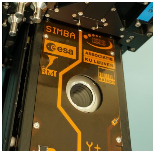
Figure 7. Location of the star tracker on the satellite close to the reflective edge of the panel on the SIMBA mission
