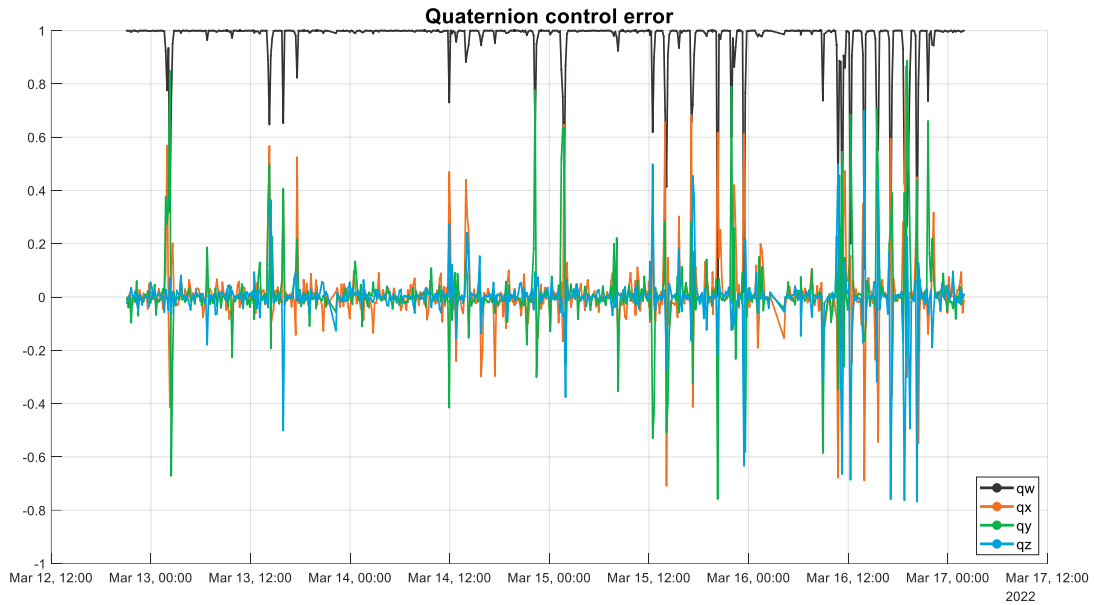
Figure 9: Steady-state quaternion control error in nadir pointing on the SIMBA mission
