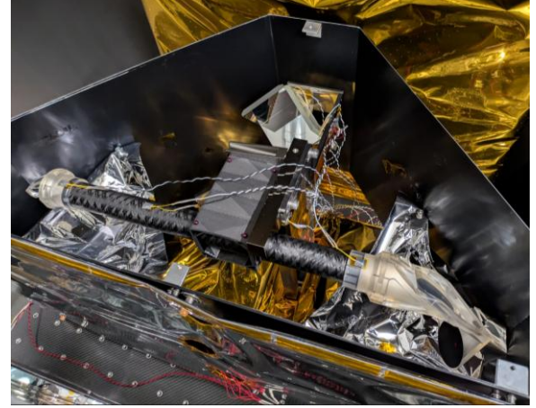
Fig. 7. Left: Test setup for the measurement of the optical path length error of the TMA. Right: Picture of the TMA FM1 with corner cube installed at the reference plate within its test enclosure.
