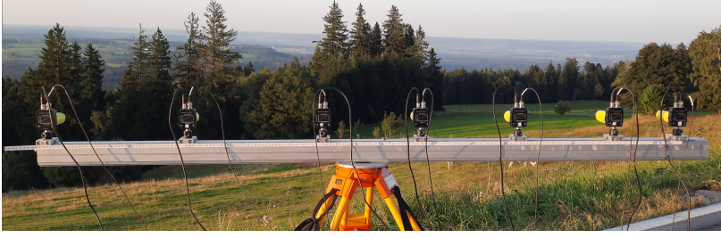
Figure 5. Receiver configuration. Seven identical photodetectors are arranged horizontally to enable the measurement of off-axis power statistics. PD0 (Figure 3) is the photodetector located furthest to the right and is used as the reference point at 0 cm (all other photodetector positions are measured relative to this point). The cables connected to the photodetectors were secured after this photo was taken to prevent misalignment due to their movement.
