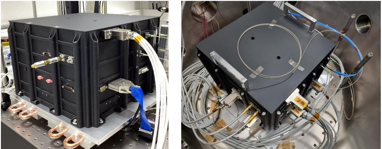
Figure 2: Fully assembled EM laser Head at STI (left) and inside the vacuum chamber at CSEM (right)
