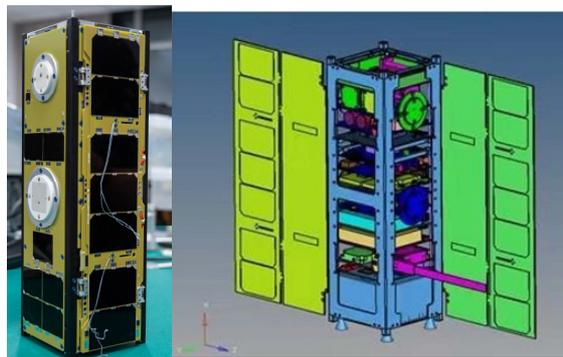
Fig. 2 SSS-2A external equipment layout.
