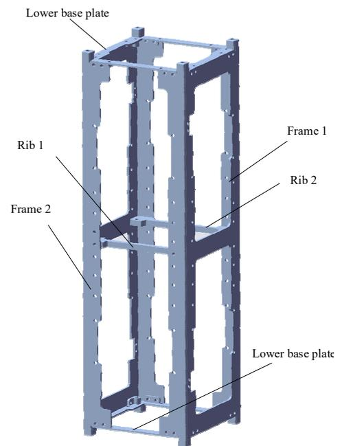
Fig.5 The SSS-2A structure
