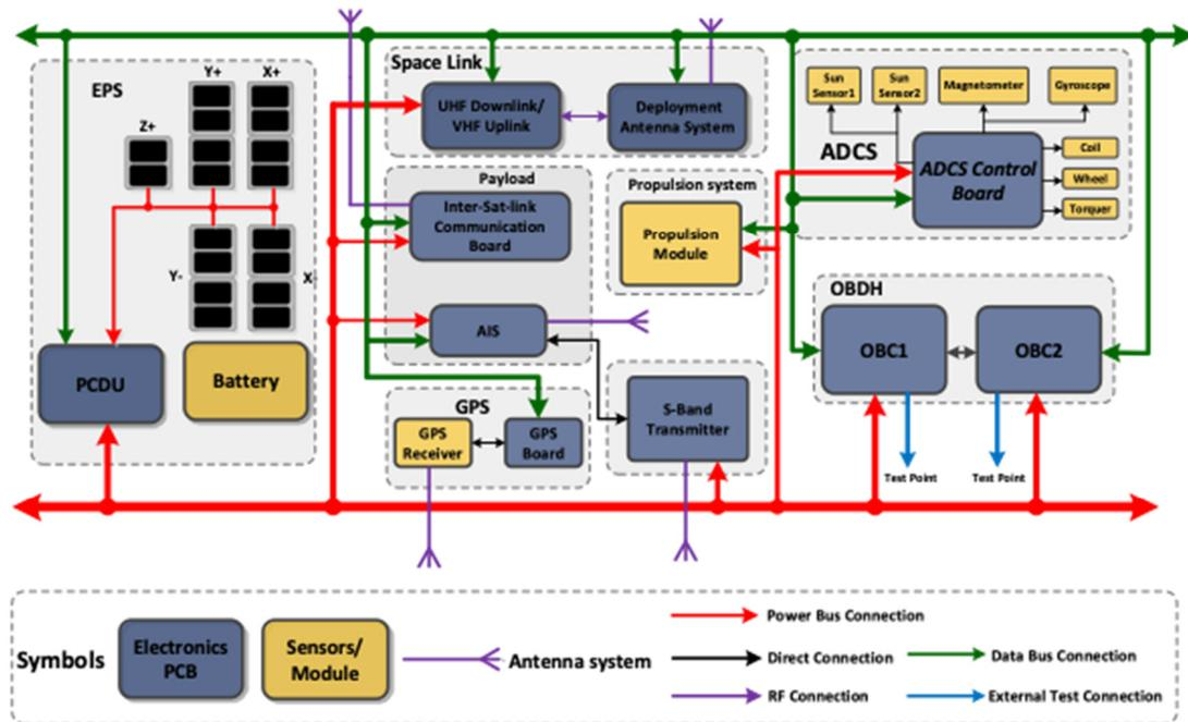
Fig.3 SSS-2A system block diagram.
