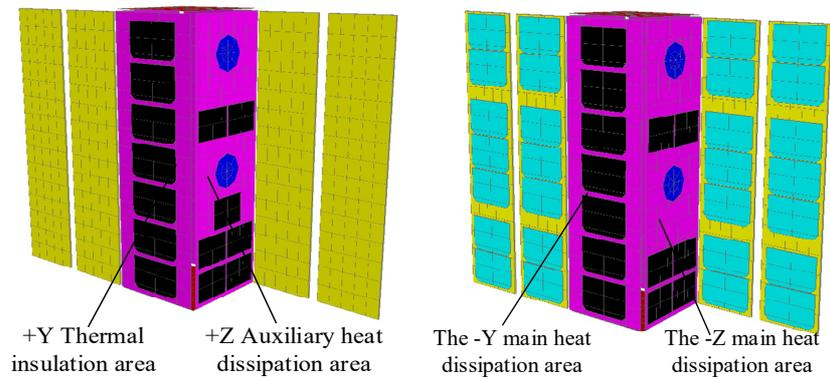
Fig. 6 Schematic diagram of satellite heat dissipation surface design
