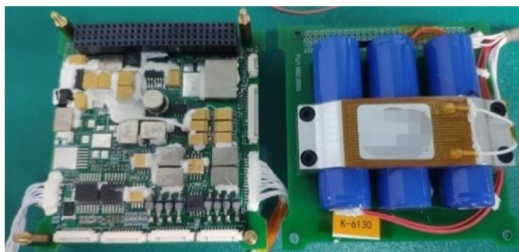
Fig.8 The electrical power system.
