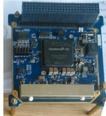
Fig.12 The AIS payload.
