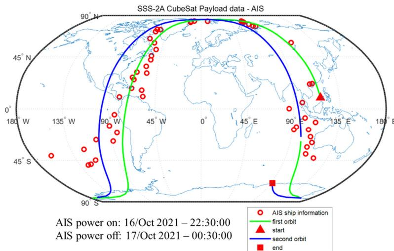
Fig.17 SSS-2A capture ship signal over two orbits
