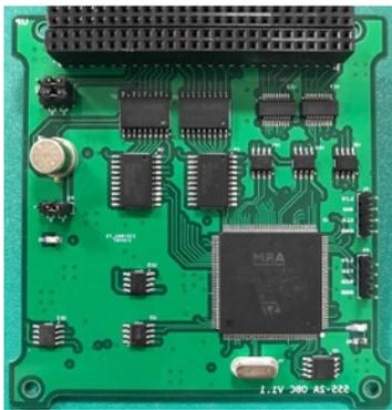
Fig.7 The on board computer.
