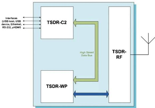
Fig.11 The inter-sat communication payload.
