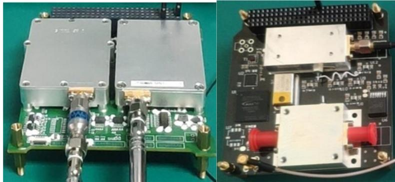
Fig.9 UHF/VHF transceiver and USB transmitter.
