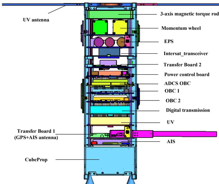
Fig.4 The layout of SSS-2A satellite
