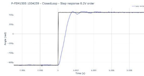
Figure 17. P-FSM150S small step resp. in Close Loop
