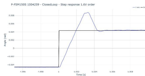
Figure 16. P-FSM150S step response in Close Loop
