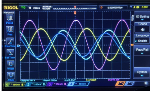
Figure 6. Left: the four raw detector signals at a heterodyne frequency of 10 kHz. Right: Amplitude spectral density of the displacement noise of the two interferometers
